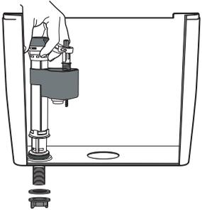
1. Insert the new fill valve with silicon seal at the base in the inlet hole of water tank and screw on the nut with collar tightly.
