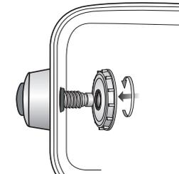
2. Insert the button into the oval hole of tank and then screw up the flanged nut in sequence.
