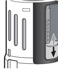
6. Adjust the half flush volume by sliding the marked part up or down. When the buoy is higher, the discharge water volume is less. Slide down the part can buoy little until you are flushing enough water.
