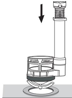
2. Put the base into the ceramic hole.
