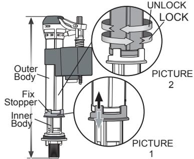
3. At the base of the fill valve's outer body, unlock the fix stopper (see picture 1) by pushing it down, then twist the outer body (see picture 2) clockwise to unlock. Adjust the outer body to the desired height. After setting it, twist the outer body counter clockwise to lock it to that position then pull the fix stopper upward to secure it.
