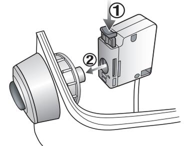
3. Push in switch box's green button (1) to connect with button body.
