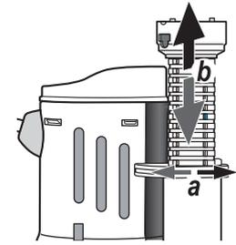
5. To adjust the height of the overflow pipe, slide the lock (a), then set the desired height of the overflow pipe (b). Put the lock back after.
