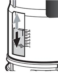
7. Adjust the full flush volume by sliding the red part up or down. When the buoy is higher, the discharge water volume is less. Slide down the part can buoy little until you are flushing enough water.
