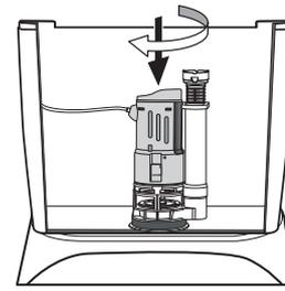
4. Take the body of flush valve and set it into the base and lock in place by rotating it clockwise.
