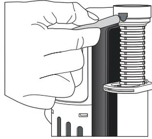
2. Connect the refill tube with refill restrictor from fill valve to the overflow pipe of the flush valve.
