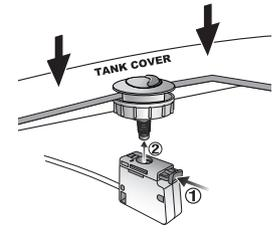
3. Push in switch box's green button (1) to connect with button body.
