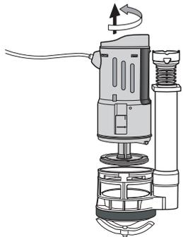
1. Hold the base of the flush valve and rotate the body counter-clockwise. Take it out from base.
